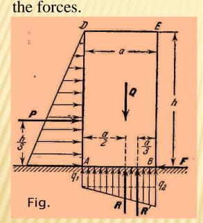
Solution. Consider a section of the dam of unit length perpendicular to the plane of the diagram. Consider further the forces acting on the section as if they were applied at the median cross section shown in Fig. These forces are: the pressure of the water P, the weight of the dam Q, the vertical reaction of the foundation, which we shall denote by two forces R and R', and the horizontal reaction F.
