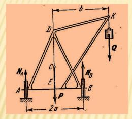
S o 1 u t i o n. Consider the equilibrium of the crane-and-load system taken as a free body: the active forces are P and Q, the unknown forces are the reactions  $N_A$  and  $N_B$  of the removed constraints.
