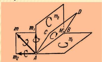
S o 1 u t i o n. Denote the moments of the two couples by vectors  $m_1$  and  $m_2$  applied at an arbitrary point A; the moment of the resultant couples is denoted by vector m.
