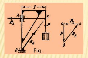
S o 1 u t i o n. To solve the problem by the graphical method draw a close triangle abc with forces P,  $R_A$ ,  $R_B$  as its sides starting with the given force P. From the similarity of triangles abc and ABE we obtain:
