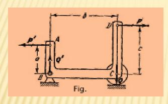
So 1 u t i o n. Replace couple (P,P') with an equivalent couple (Q,Q') whose two forces are directed along the reactions of the constraints. The moments of the two couples are equal, i.e., P(c-a)=Qb, consequently the loads on the constraints are:  $Q = Q' = \frac{c-a}{b}P = 50N$
