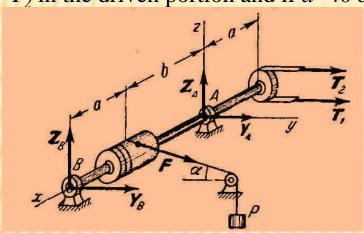
S o l u t i o n. As the shaft rotates uniformly, the forces acting on it are in equilibrium and the equations of equilibrium can be applied.
