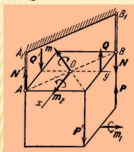
S o l u t i o n. The system of couples (P, P') and (Q, Q') is equivalent to a couple and can be balanced only by a couple. Hence, the required reactions N and N' must form a couple.
