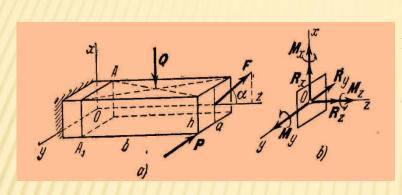
Solution. For this reduce all the forces to the centre *O* of the section, and place the origin of the coordinate system there.
