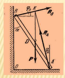
S o 1 u t i o n. Let us examine the position of impending slip of the ladder by graphical method. For impending motion the forces acting on the ladder are the reactions of the floor and wall  $R_A$  and  $R_B$  which are inclined at the angle of friction  $\varphi_0$  to the normals of the surfaces. The action lines of the reaction intersect at K.
