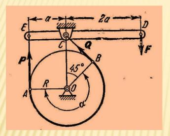
S o l u t i o n. Acting on the drum and band AB wrapped around it is a force P (evidently P=2F) applied at A and a force Q applied at B.
