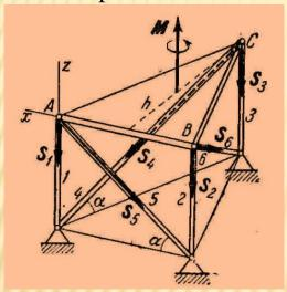
S o 1 u t i o n. Regarding the plate as a free body, draw, as shown in the figure, the vector of moment M of the couple and the reactions of the bars  $S_1, S_2, ..., S_6$ .
