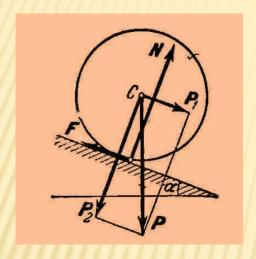
S o 1 u t i o n. Consider the position of impending motion, when  $\alpha = \alpha_l$ .
