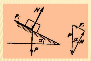
S o 1 u t i o n. The problem requires that all possible positions for the equilibrium of the load be determined. For this, let us first establish the position of impending motion at which  $\alpha = \alpha_l$ . In that position acting on the load are its weight P, the normal reaction N and the limiting friction  $F_l$ .
