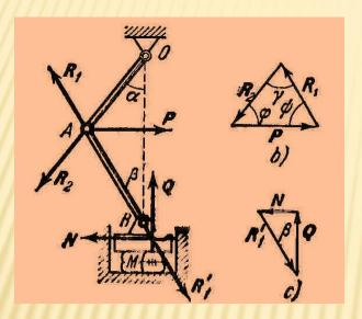
Solution. First consider the equilibrium of the hinge A to which the given force P is applied. Regarding the hinge as a free body, we find that also acting on it are the reactions  $R_1$  and  $R_2$  of the rods directed along them. Construct a force triangle (Fig.b). Its angles are  $\varphi=90^{\circ}-\alpha$ ,  $\psi=90^{\circ}-\beta$ ,  $\gamma=\alpha+\beta$ . By the law of sines we have:
