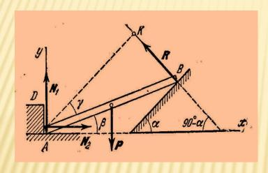
S o 1 u t i o n. Consider the equilibrium of the beam as a free body. Acting on it are the given force P and the reactions R,  $N_I$ , and  $N_2$  of the constraints directed normal to the respective surfaces. Draw the coordinate axes and write the equilibrium equations, taking the moments about A.
