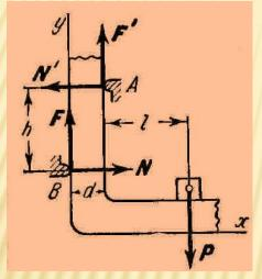
S o 1 u t i o n. Let us denote the weight of the load by P and its distance from the vertical member of the bar by l. Now consider the position of impending slip of the bar, when  $d = d_l$ . In this position acting on it are force P, N, F, N', and F', where F and F' are the forces of limiting friction.
