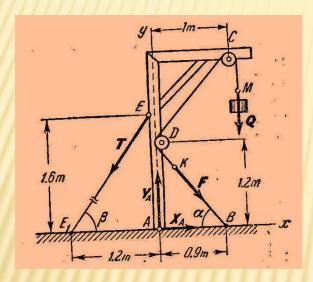
S o 1 u t i o n. Consider the whole system of the frame and the portion KDCM of the string as a single free rigid body. Acting on it are: the weight Q, the tension F in section DB of the string, the reactions T,  $X_A$ , and  $Y_A$  of the constraints. The internal forces cancel each other. As the friction of the pulleys is neglected F = Q.
