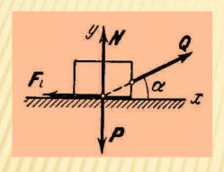
S o 1 u t i o n. According to the conditions of the problem we have to consider the position of impending motion of the load. In this position acting on it are forces P, Q, N and  $F_l$ . Writing the equilibrium equations in terms of the projections on the coordinate axes, we obtain:
