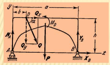
S o l u t i o n. In this problem it is more convenient to use eqs., taking the moments about A and B and the force projections on axis Ax, and each equation will contain one unknown force.
