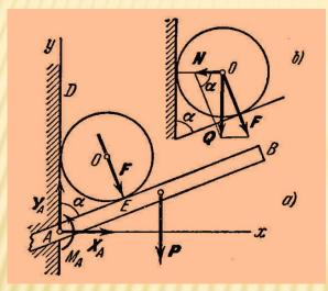
Solution. Consider the equilibrium of the beam as a free body. Acting on it are force P applied halfway between A and B, force F applied perpendicular to the beam at E (but not force Q, which is applied to the cylinder, no to the beam!), and the reactions of the embedding, indicated by the rectangular components  $X_A$  and  $Y_A$  and a couple of moment  $M_A$ .
