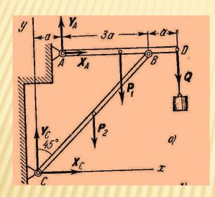
Solution. Considering the bracket as a whole as a free body, we find the acting on it are the given forces  $P_1$ ,  $P_2$ , Q and the reactions of the supports  $X_A$ ,  $Y_A$ ,  $X_C$ ,  $Y_C$ . But with its constraints removed the bracket is no longer rigid body, because the members can turn about pin B. On the other hand, by the principle of solidification, if it is in equilibrium the forces acting on it must satisfy the conditions of static equilibrium.
