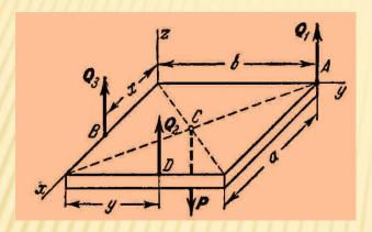
S o l u t i o n. The plate is a free body acted upon by four parallel forces  $Q_1$ ,  $Q_2$ ,  $Q_3$  and P, where P is the weight of the plate.
