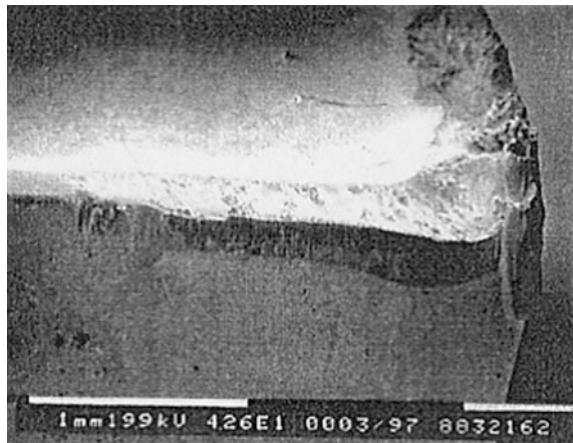
Fig. 2 Damaged cutting tool edge in machining Ti-6Al-4V alloy at speed and feed of 100 m/min and 0.25 mm/rev, respectively [47]
