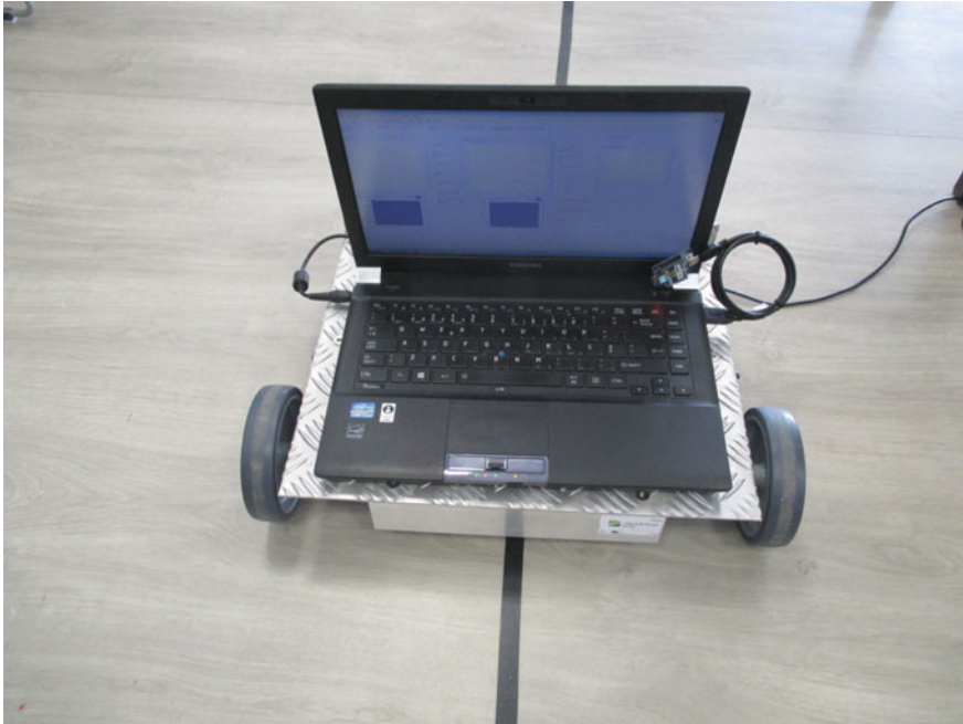
Fig. 27 AGV performing path tracking (in-door test)
