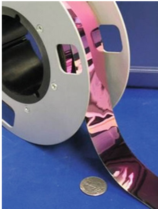
Fig. 11.24 Superconducting metal matrix composites: (a) first generation high temperature superconductor (HTS) filaments in a silver matrix (in commercial production), (b) second generation coated conductor composite, consisting of a superconductor layer, coated with a noble metal, on an alloy substrate (Courtesy of J. Jackson, American Superconductor)
