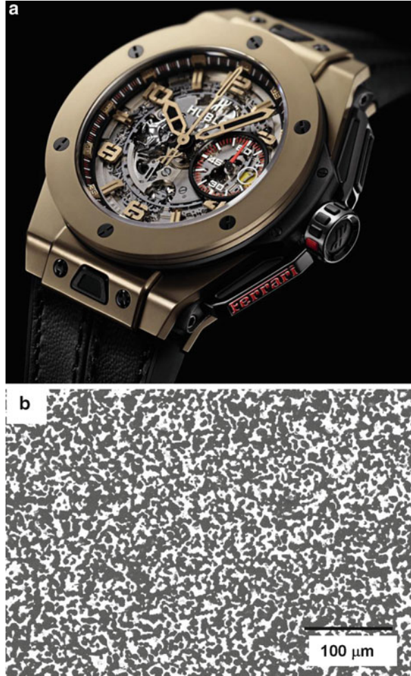
Fig. 11.30 (a) B_4C particle reinforced gold matrix composite watch casing and (b) 3D network microstructure of the composite, where bright is gold matrix and dark is B_4C . The volume fraction of reinforcement is 70 % (Courtesy of S. Hasanovic, Hublot)
