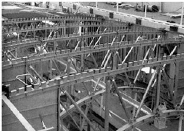
Fig. 11.10 Al/B f tubular struts in the frame and rib truss members of the mid fuselage section of the space shuttle (Courtesy of S. Rawal, reprinted with permission from The Minerals, Metals, and Materials Society). The struts provide a weight savings of 45 % over unreinforced aluminum
