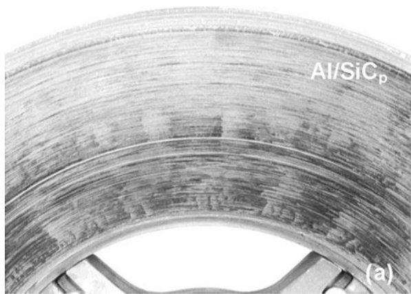
Fig. 11.19 Thermal cracking behavior in (a) Al/SiC p and (b) steel after wear testing (Courtesy of H. Ruppert). The steel brake shows significant amount of cracking ( white lines ) while the MMC is in relatively good condition
